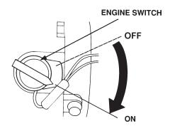
Figure 13. Engine ON/OFF Switch
